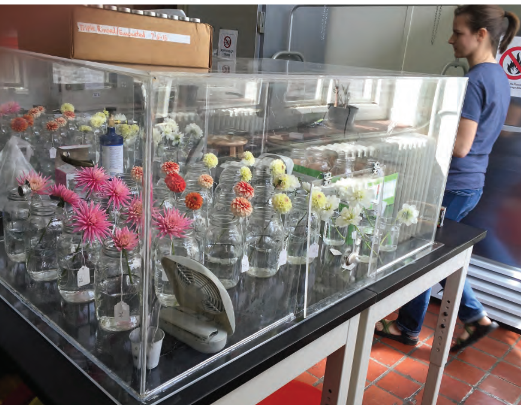
Ethylene treatment chamber.
